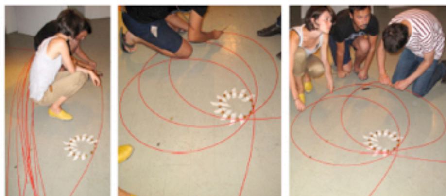
Fig. 5 Assembling of fiberglass wire modules into knotted structure
